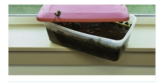
Within 3–10 days, the MFC will generally produce enough power to make the LED blink; the more power, the faster the blinking. Keep your MFC warm and moist inside to help the bacteria grow and produce the most power.
