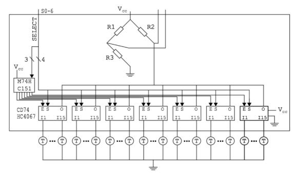
Figure 2 – The multiplexer board and Wheatstone bridge.
