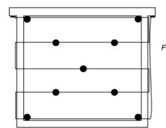
Figure 1 – A frame of the beehive with nine thermistors on the metal wire.
