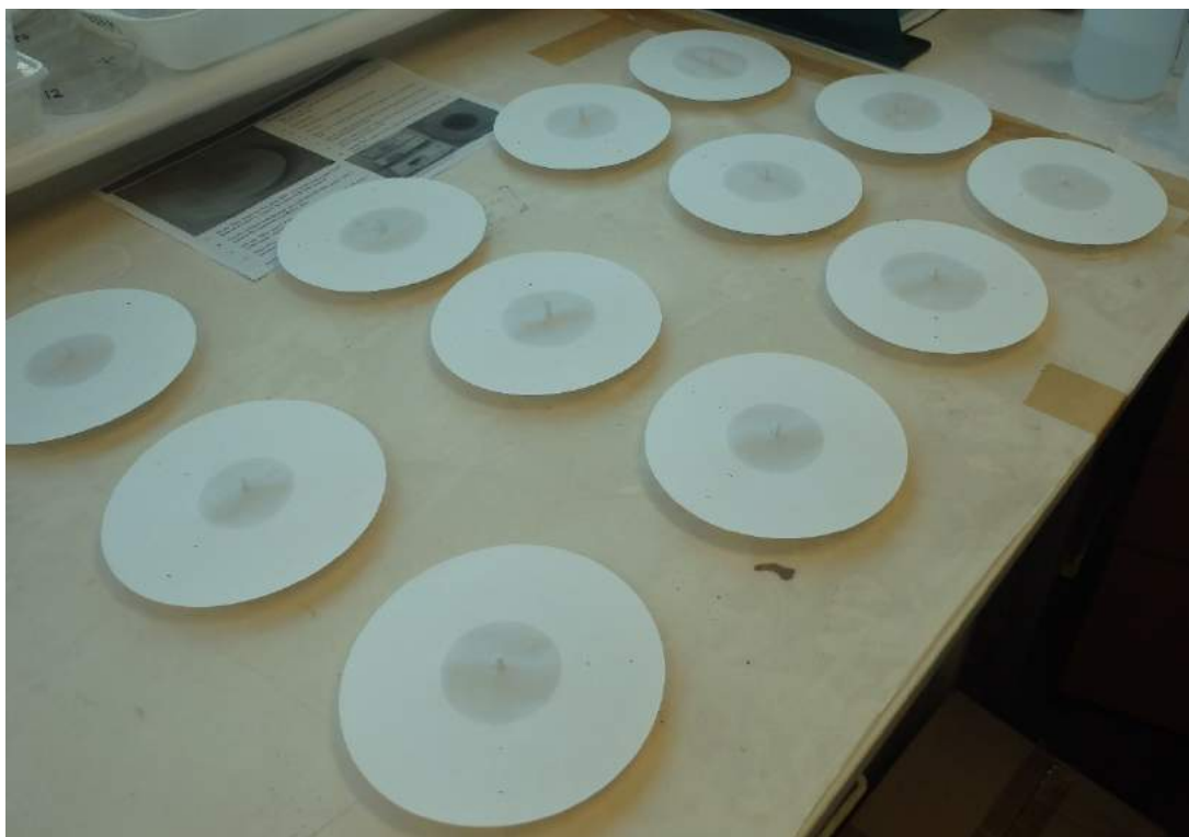
Figure 2.3. Filter papers being prepared with silver nitrate solution.
