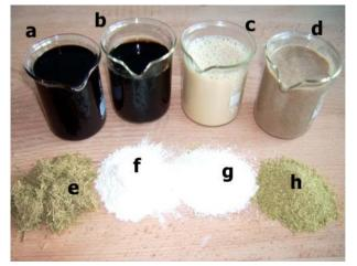
Fig. 4: Used materials: a-Phenol resin, b-PLA semi product, c, d-plants rests of glucose production, e-fibre, f-starch, g-cellulose, h-raps pressed cake
