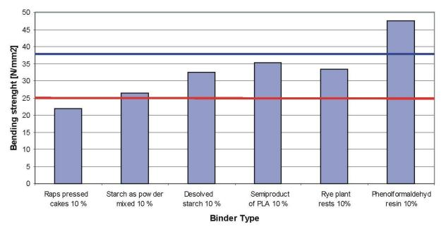
Fig. 6: The bending strength of natural fibreboard with different binders (material: hemp silage mixed with wooden fibre 6:4, density 1140 kg/m<sup>3</sup>, thickness 10mm). — minimum required strength towards EN 622-2 for HDF boards for common purposes in dry area, and — for highly reliable boards for construction purposes in moist area.
