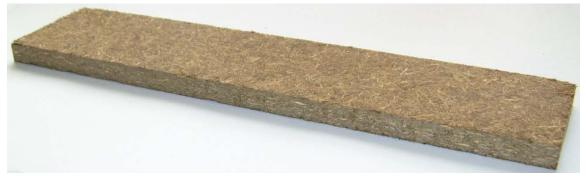
Fig. 5: Fibreboard (bending test sample) made of preserved hemp (thickness 10 mm, density 500-1200 kg/m<sup>3</sup>, pressing temperature 200 °C, pressing time 6 min.)
