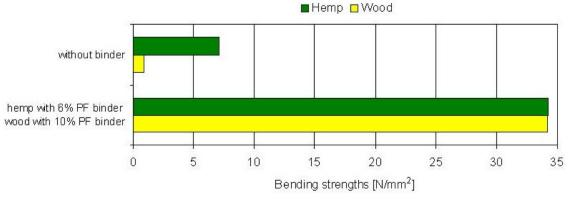
Fig. 7: The bending strength of fibreboard made of hemp and wood fibre (thickness 10 mm, density 790 kg/m<sup>3</sup>, pressing time 6 min., binder PF resin)
